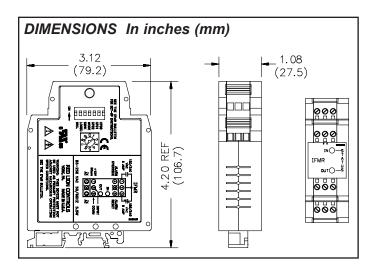
CAUTION: Risk of Danger. Read complete instructions prior to installation and operation of the unit. The IFMR operates in one of six output modes, as selected by the user. The programmable Minimum Response Time provides optimum response vs. input filtering for any input frequency. The offset and hysteresis settings provide flexible adjustment of the relay trip and release points.
